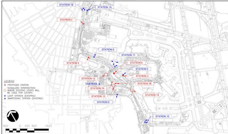
TrafInfo Communications, Inc. has been under contract by the Massachusetts Port Authority (Massport) since 2001 to provide operations and maintenance of their Automatic Traffic Monitoring System (ATMS) equipment on the Logan International Airport terminal area roadways.
